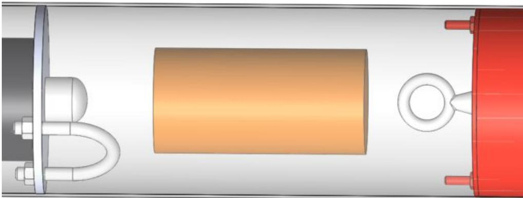
Figure 3.5.1. - Representation of Drogue Chute Inside Rocket
