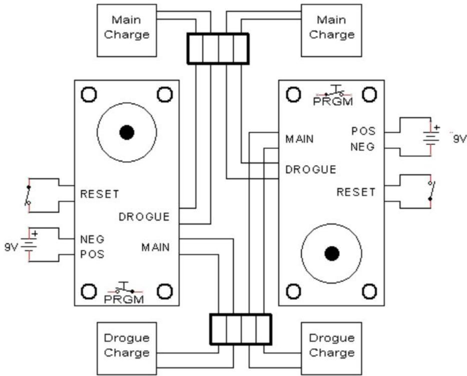
Figure 3.10.3: Dual Redundant System
