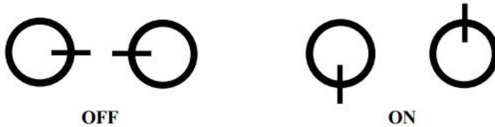
Figure 5.4.1. Altimeter On/Off Configurations.
