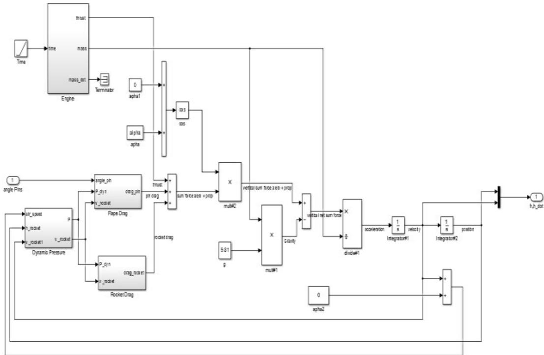
Figure 4.2.2. Simulink Model for Rocket Block
