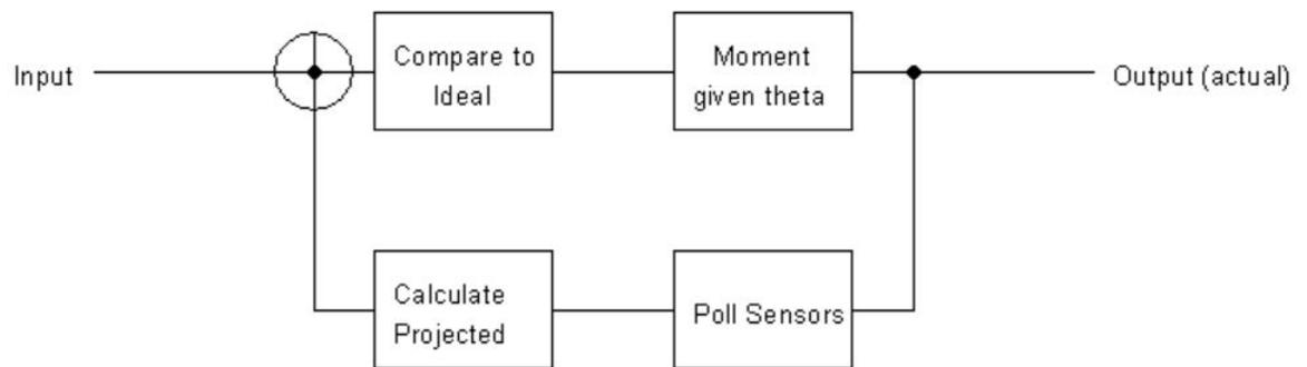
Figure 4.5.1 Control system block diagram and logic flow
