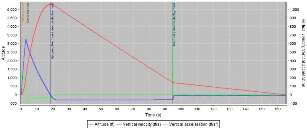
Figure 3.14.1 Full Scale Simulation
