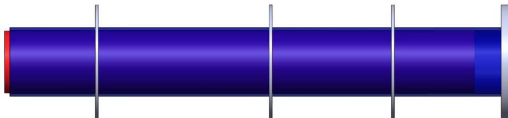
Figure 3.11.1 Motor and Center Rings
