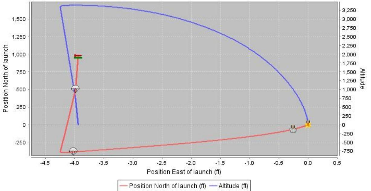
Figure 3.13.2. Drift Profile Windspeed at 5 mph
