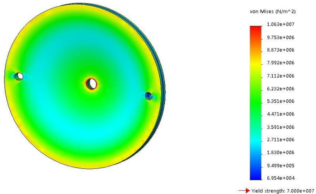
Figure 3.7.1 - Load Analysis on Bulkhead
