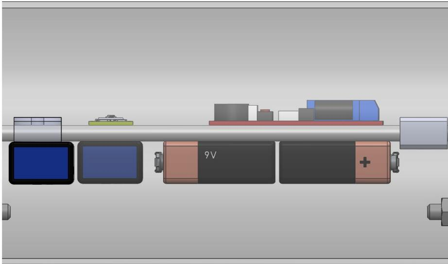
Figure 3.6.3 - Tray With Mounted Hardware
