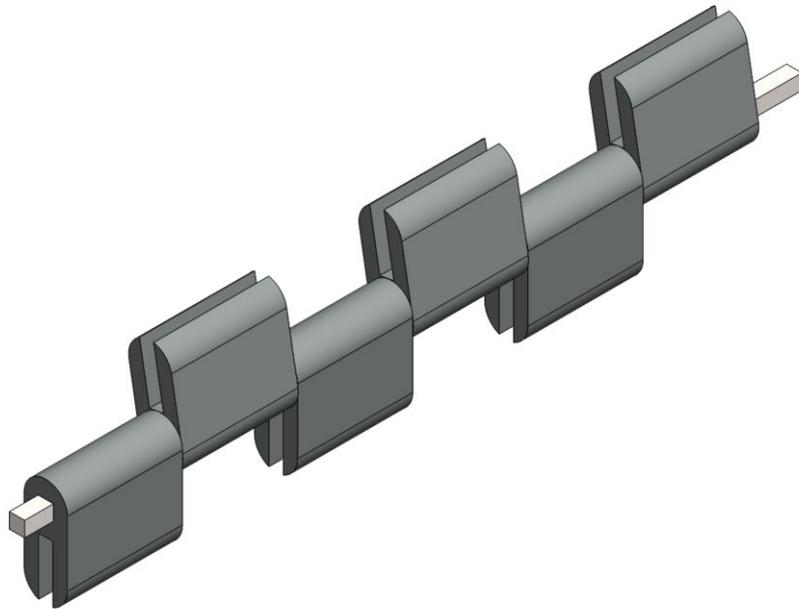
Figure 3.2.3 Hinge Assembly
