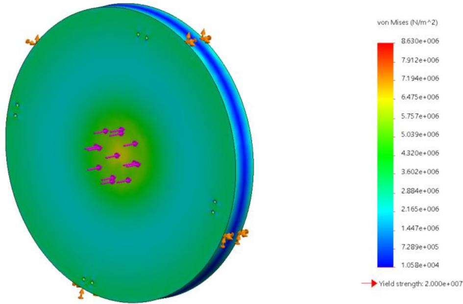
Figure 3.3.2. - Load Analysis on Thrust Plate
