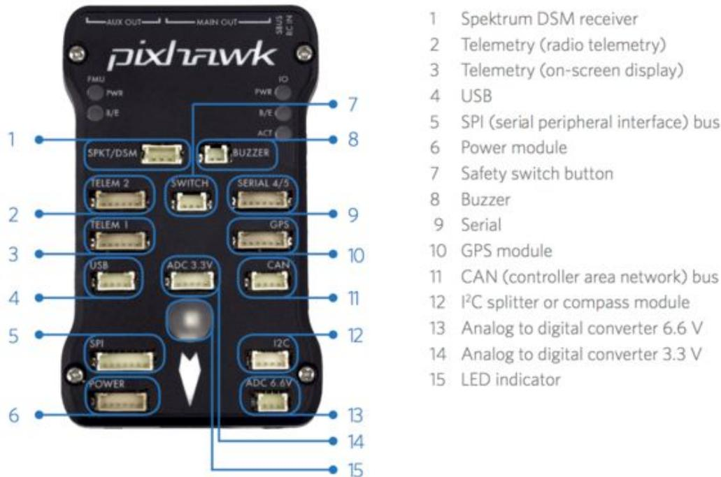
Figure 4.1.1 Pixhawk autopilot flight controller
