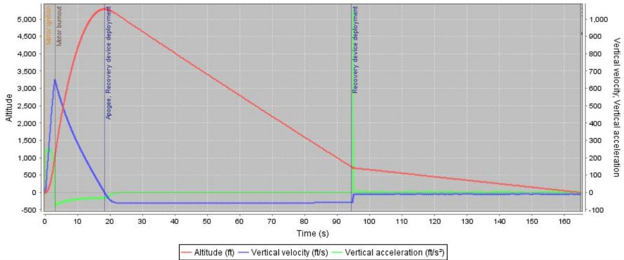
Figure 3.14.1 Full Scale Simulation
