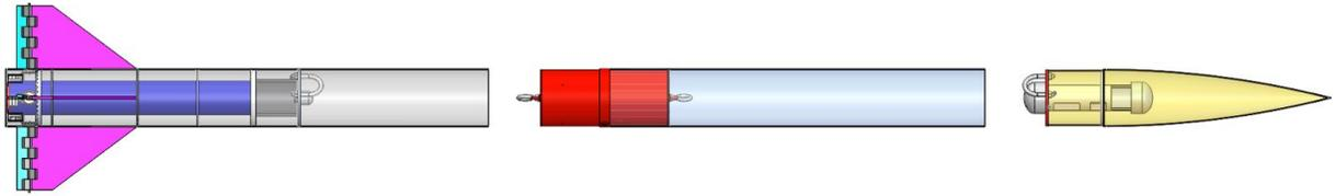
Figure 3.1.2. Figure Showing Separation of Sections
