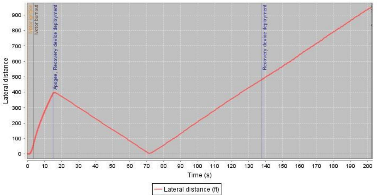
Figure 3.13.3. Lateral Distance Windspeed at 5 mph
