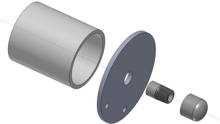
Figure 3.4.1 - Exploded View of MAS
