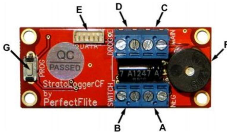
Figure 3.10.1: The StratologgerCF altimeters with connection labels (for reference)
