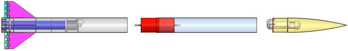
Figure 3.1.2. Figure Showing Separation of Sections
