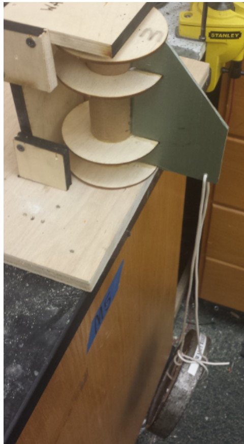
Figure 22: Fin Test Jig and Test Article
