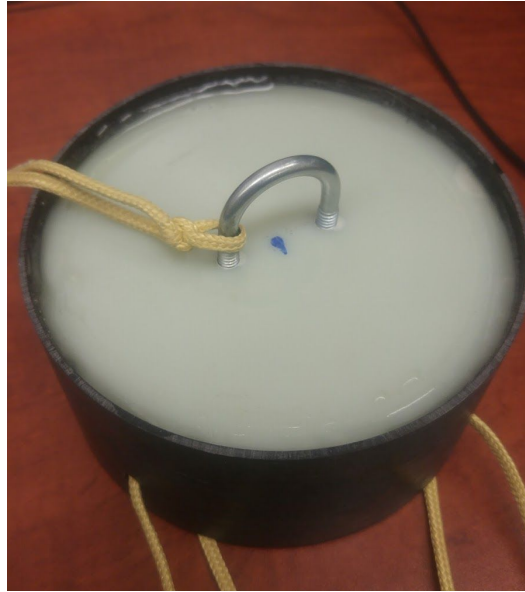
Figure 3.8.1 Bulkhead after epoxy
