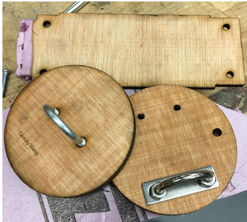
Figure 3.9.3: Prototyped Avionics Bay using Laser Cutter
