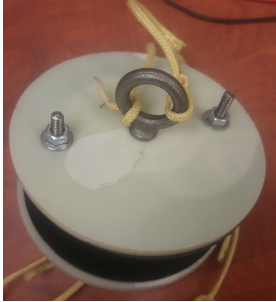
Figure 3.8.3 Bulkhead with Hole Locations
