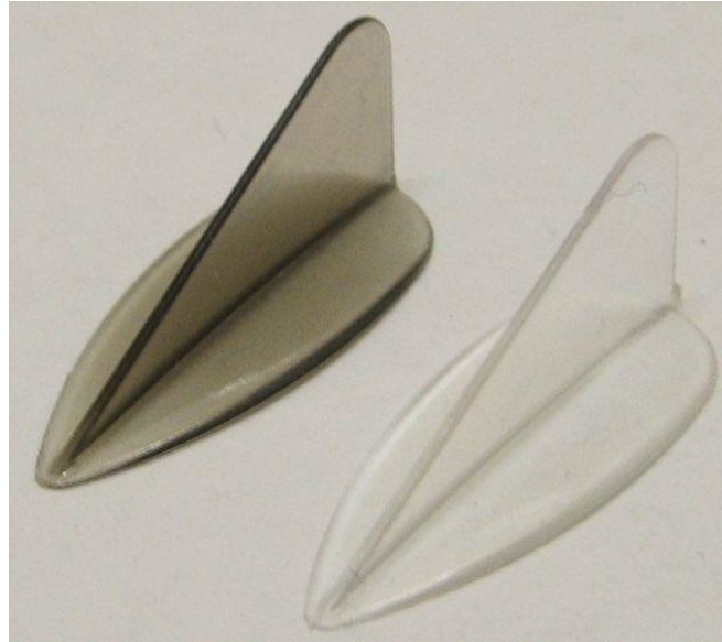
Figure 11: Concept Airbrake Fin Design with sanded edges for improved drag and maximum usable surface area
