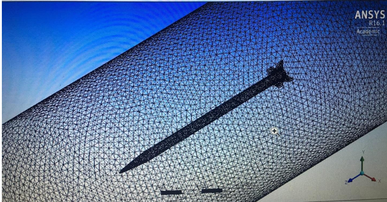
Figure X. Mesh around launch vehicle body
