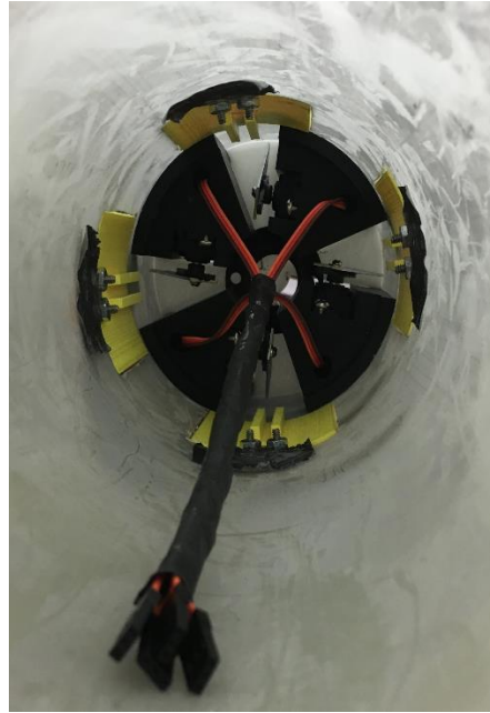
Figure 24: Servo and Servo Mount Placement
