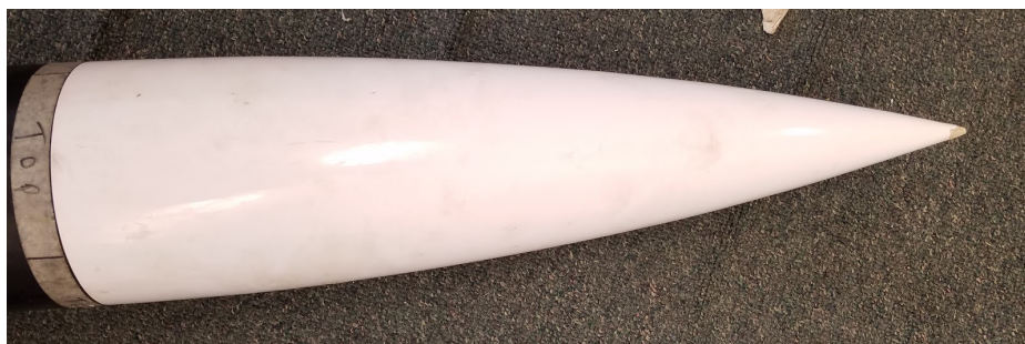
Figure 3.1.9: Actual image of the Nose Cone
