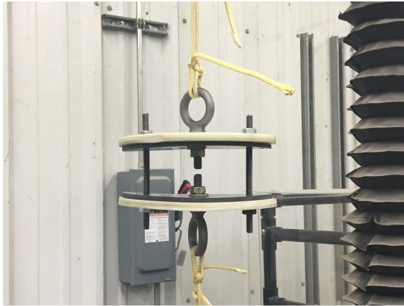
Figure 8.1.7. Deformation of fiberglass bulkheads
