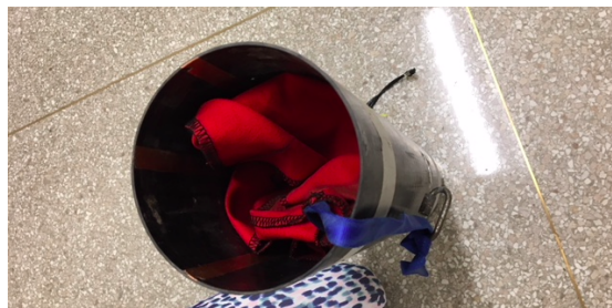
Figure 3.2.26 Packed Drogue Parachute
