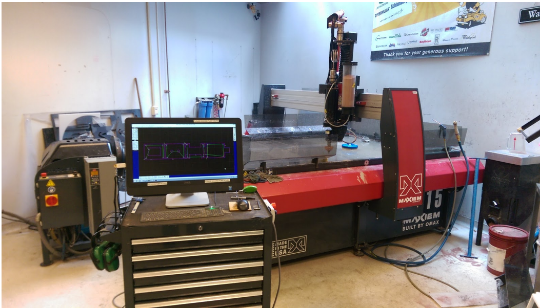
Figure 3.1.27 Maxiem 1515 Waterjet cutter
