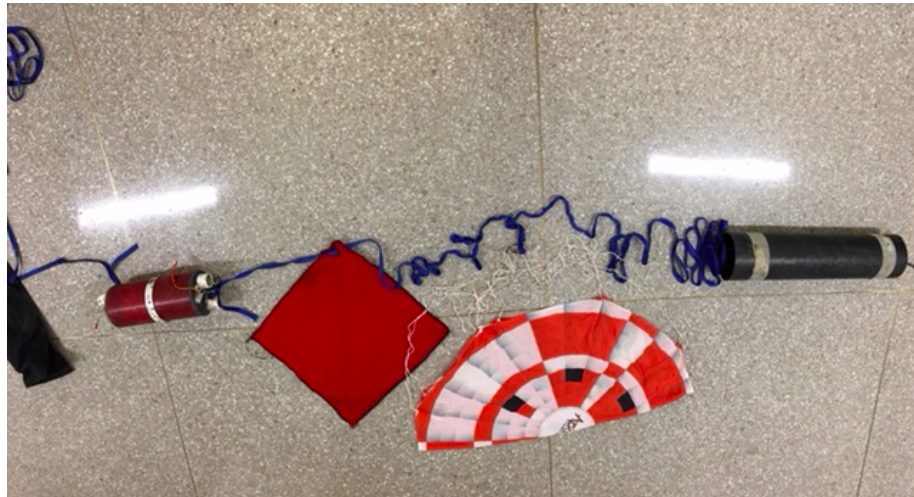
Figure 3.2.25 Drogue Parachute Layout
