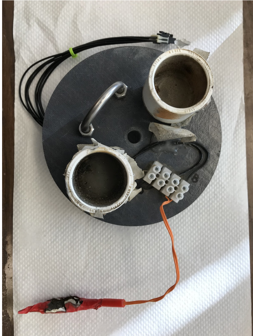
Figure 3.1.26 Bulkhead with connector joined to terminal blocks
