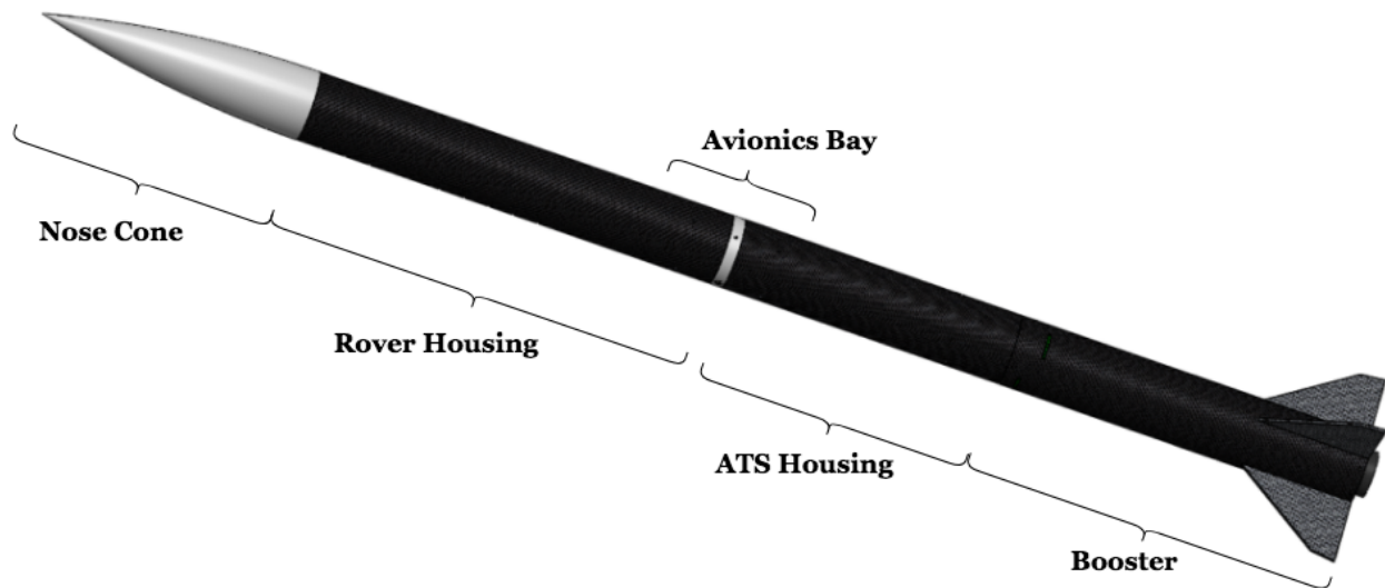
Figure 3.1.1: Sections of Full Scale Launch Vehicle
