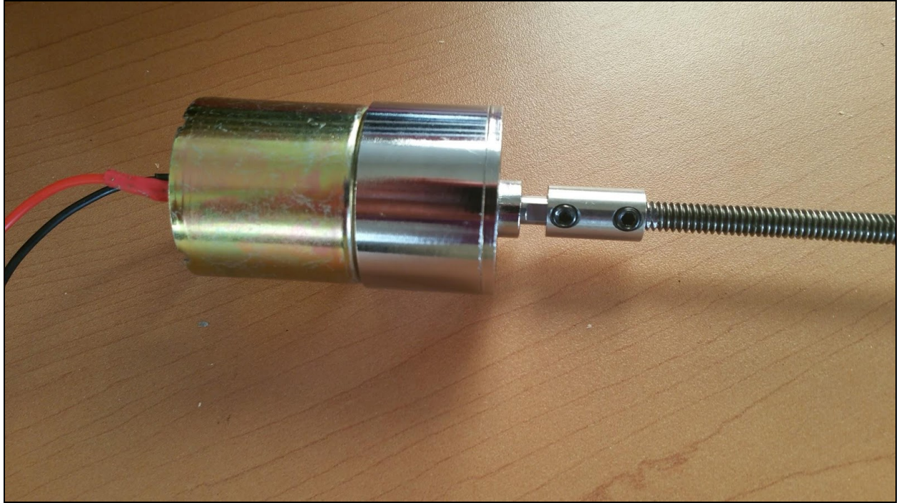
Figure 6.2.3. The motor, shaft coupler, and threaded rod used in the subscale prototype
